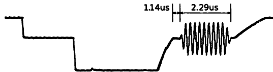
Figure 16-1: "Colour Burst" synchronisation - 10 cycles of sub-carrier
